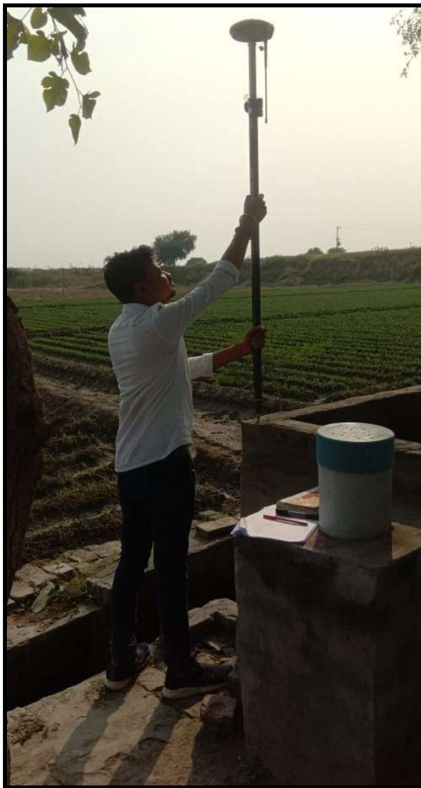
PHOTOGRAPH 13: Temporary benchmark creation in Beas River, Tarn Taran.
