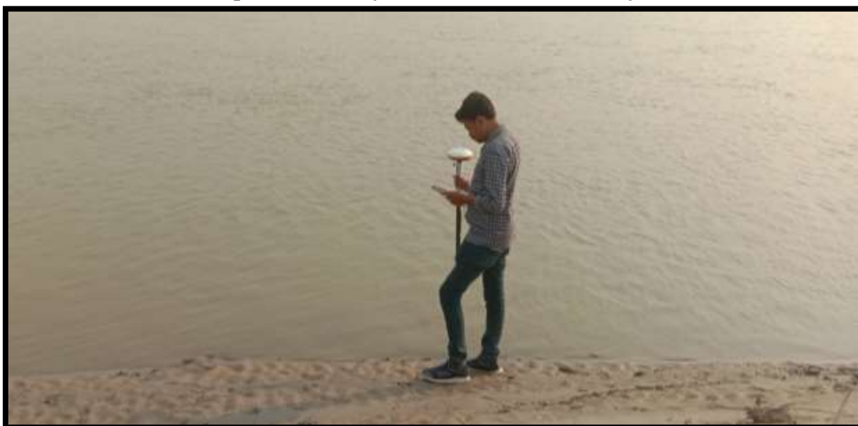
PHOTOGRAPH 4: DGPS survey for determining Thalweg point of River Sutlej, Tarn Taran.
